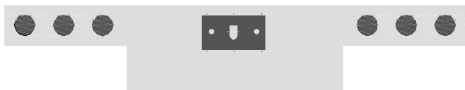
Rear T-Bar with (6) 4 in. Round Light Holes and Recessed Airline Box with Trailer Air & (1) 7-Way IC975005-14
